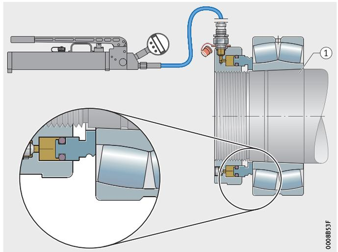
① Pressing into place on an adapter sleeve
