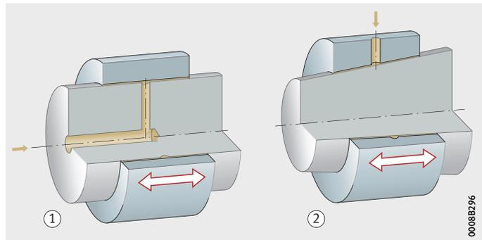
In both cases, oil grooves and feed ducts as well as threaded connectors for the pressure generation devices must be provided. The width of the oil groove is dependent on the bearing width, *Figure 6*. Further design guidelines are given in the FAG publication WL 80102, Hydraulic Method for the Mounting and Dismounting of Rolling Bearings. Hydraulic nuts are used as a mounting tool. Pressure can be generated using hand pumps and hydraulic units. In isolated cases, oil injectors can also be used.
