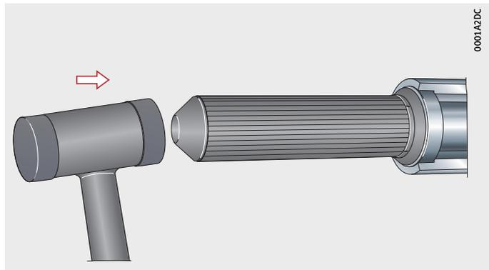
When the bearing is slid onto the taper, the inner ring is expanded and the radial internal clearance is thus reduced. The reduction in radial internal clearance is therefore valid as a measure of the seating of the inner ring.
