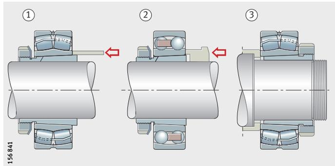
The dismounting of large bearings located using a withdrawal sleeve requires considerable force. In this case, locknuts with additional pressure screws can be used, *Figure 8*. A disc must be inserted between the inner ring and the pressure screws in order to prevent damage to the bearing.
