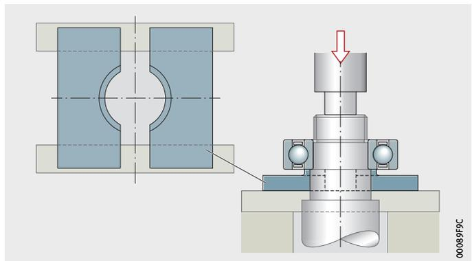
Dismounting is made much easier if the design includes extraction slots so that the extraction tool can be applied directly to the bearing ring with a tight fit. A further alternative to dismounting of bearings is the use of extraction screws.
