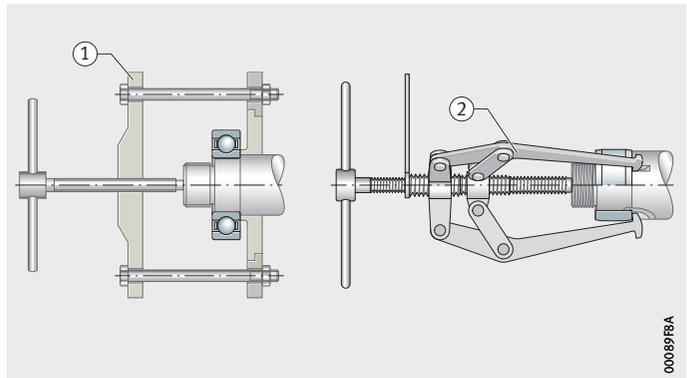
A press can also be used to assist in dismounting. It must be ensured in this case that the bearing is abutted on its inner ring in order to avoid damage. In the pressing operation, the shaft is withdrawn from the bearing.
