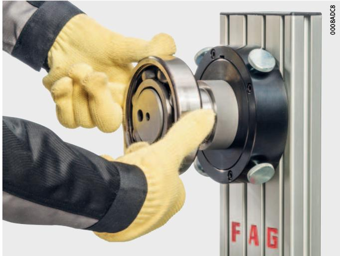
Once the inner ring has been slid in place, it must immediately be secured against its axial abutment point and held under tension until it has cooled, so that it then remains in full contact. There must not be any gap between two rings positioned adjacent to each other.
